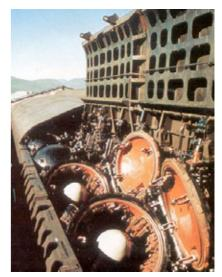
Torpedo munitions comprised 24 torpedoes held in open rack magazines, potentially including torpedoes of nuclear capability, firing from 2x650mm and 4x533mm torpedo tubes in the bow (No 1) compartment. The armaments could also include ASW Harpoon-type rockets and seabed mines also deployed from the forward torpedo tubes.
